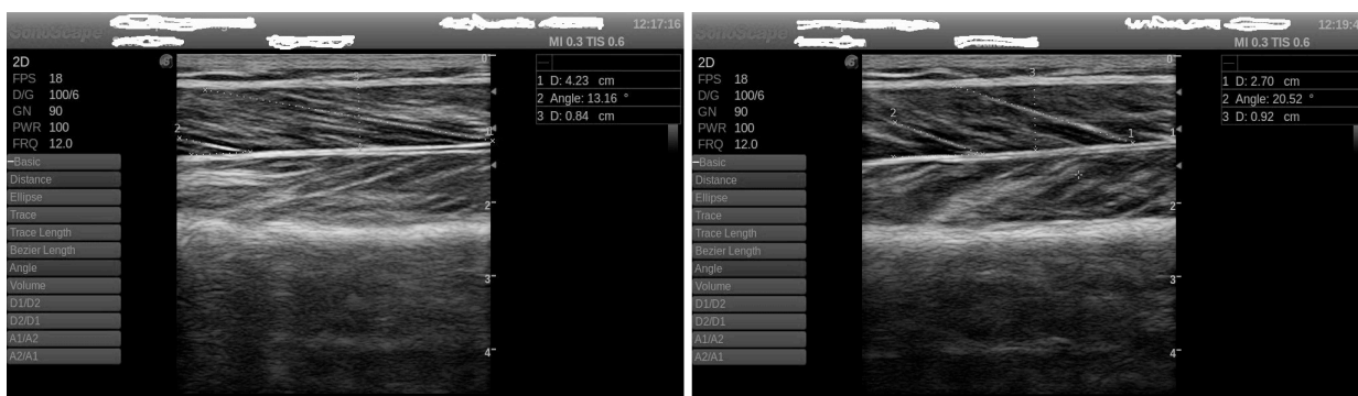
Figure 3. Ultrasonographic imaging of the peroneus longus muscle demonstrating the measurement of muscle thickness, fascicle length, and pennation angle in (a) relaxed and (b) contracted condition.
