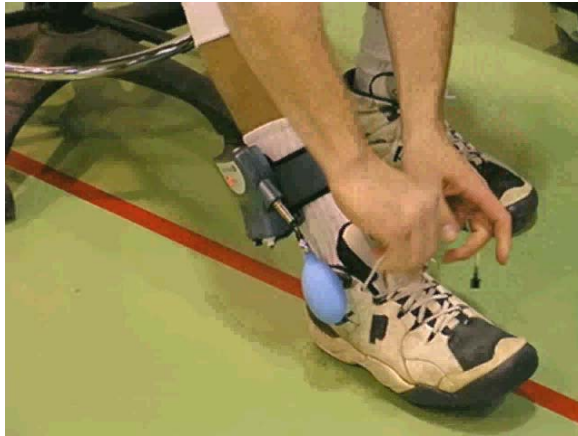
Fig. 1. The computerized air-insole auditory biofeedback system
